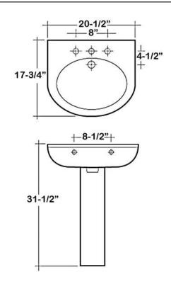
Dimensions of fixture are nominal and may vary within the range of tolerances established by ASME Standard A112.19.2-2013. Dimensions and specifications subject to change without notice.
